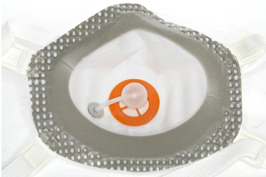
Fig. 8 Filtering facepiece fitted with 'ball' sample probe
