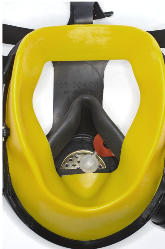
Fig. 10 Full face mask fitted with 'ball' sample probe
