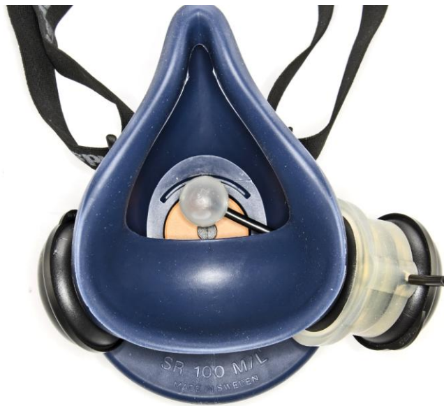
Fig. 9 Half mask fitted with 'ball' sample probe
